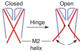
**Figure 4.40** Schematic illustration of the hinge-bending model for the opening of the bacterial KcsA channel. The M2 helices from each subunit bend outward at a specific glycine residue, which opens the gate at the intracellular end of the channel to K<sup>+</sup> ions. (REPRINTED BY PERMISSION FROM MACMILLAN PUBLISHER LTD: FROM B. L. KELLY AND A. GROSS, NATURE STRUCT. BIOL. 10:280, 2003; COPYRIGHT 2003.)
