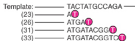
Tube 4: Products of ddT reaction
