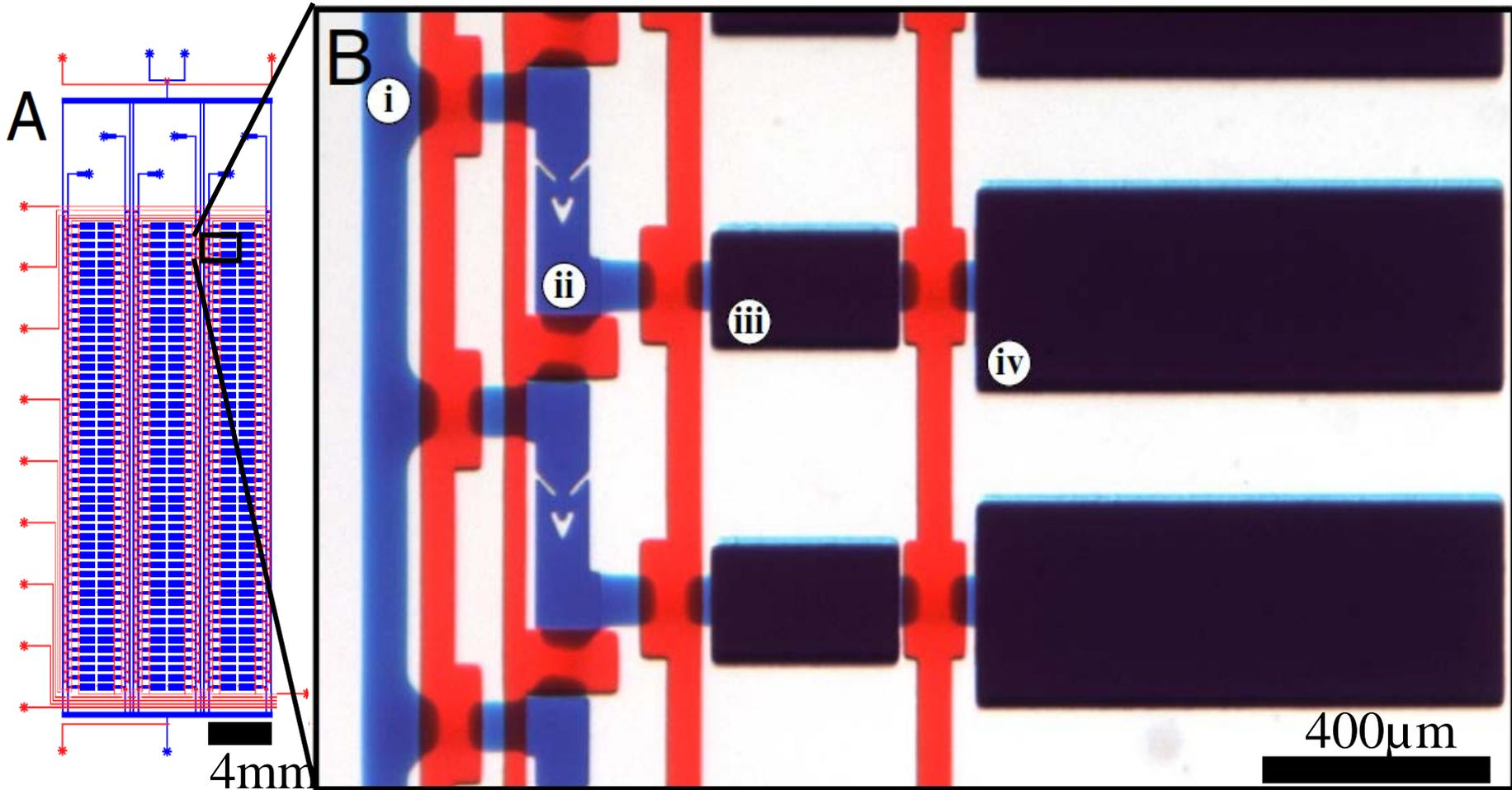
Each unit consists of (i) a reagent injection line, (ii) a 0.6-nL cell capture chamber with integrated cell traps, (iii) a 10-nL reverse transcription (RT) chamber, and (iv) a 50-nL PCR chamber.
