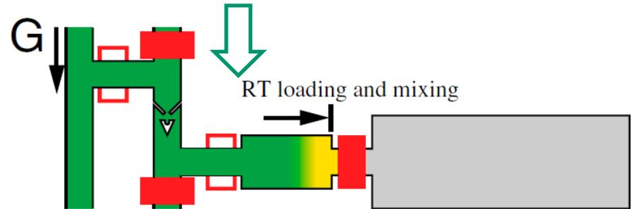
A pulsed temperature RT protocol was carried out by placing the microfluidic device on a flatbed thermocycler (2 min at 16  $^{\circ}\text{C}$ , followed by 60 cycles of 30 s at 20  $^{\circ}\text{C}$ , 30 s at 42  $^{\circ}\text{C}$ , and 1 s at 50  $^{\circ}\text{C}$ ). RT enzyme was inactivated at 85  $^{\circ}\text{C}$  (5 min), and then the device was cooled to 4  $^{\circ}\text{C}$ .
